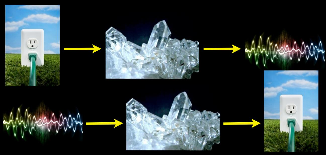
• Piezoelectric effect: the charge which builds up in certain solids in response to applied mechanical strain
