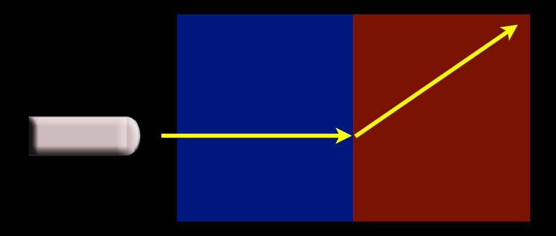
Direction of sound is changed at interface between different media
